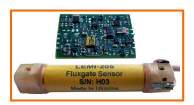
Miniature fluxgate magnetometer LEMI-205 is intended for measurements of one component magnetic field.
