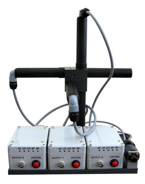
Three axis search-coil magnetometer LEMI-150 is intended for the measurements of the three orthogonal components of magnetic field fluctuations. Every individual sensor that constructs the 3D sensor is independent. There is an option to take out the individual sensor for independent use with or without its matching circuits and filters (modularity). There is an option to work with less than three sensors.
