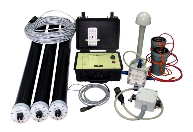
Wide band magnetotelluric station LEMI-423 is intended for the study of natural electromagnetic fluctuations in field conditions in wide temperature range. The station registers and digitizes automatically the data from 3 search-coil magnetometers and 2 electric channels. The electric channels include lightning protection unit, one of two
